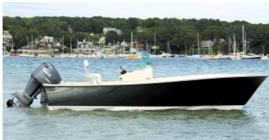
The Gloucester 20's attractive sheerline adds to the aesthetics of her profile, but it also creates a larger entry to combat chop.
